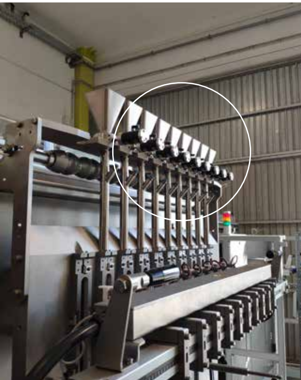
K (linear pneumatic vibrator) - Hopper emptying
