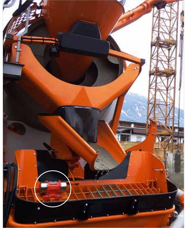
MVE-DC (electric vibrator) - Concrete pump
